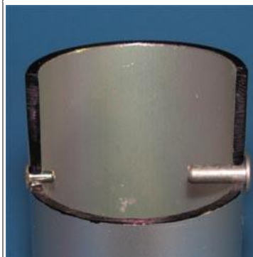
1/8" & 3/16" eyelets using the shell from a pop rivet. Use only for thru line.
