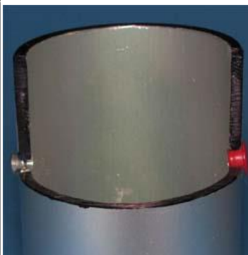
Eyelets do not protect the line from the inside edge
