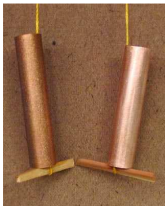
Cleaned and ready for the process. The tube on the left has been sanded with 150 grit sand paper while the right hand tube has been cleaned with steel wool
