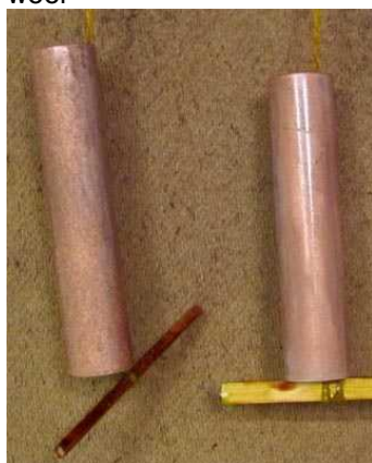
First coat of toilet bowl cleaner containing hydrochloric acid has been applied. Dried in about two days
