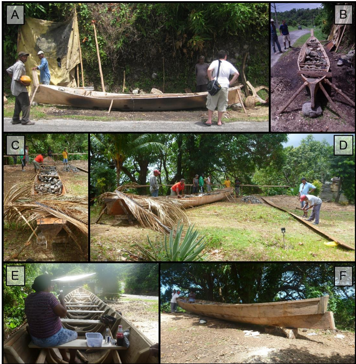
Figure 6-9. Images of two Kalinago dugout canoes being constructed. A) Side view of the small canoe built in the village of Boetica in 2009. B) View of the same canoe with rocks and water left inside to help spread the walls. C) The same view and the same process but for the much larger canoe built in Kalinago territory in 2013. D) Side view of the same canoe with workers shaping the bordage that will be attached to the side of the dugout to raise the walls, technically making this a pirogue instead of a canaoa (McKusick 1960a). E) Regina, who taught us much about this canoe, sitting in the near-finished product. F) Side view of the near-finished 38-foot canoe.
