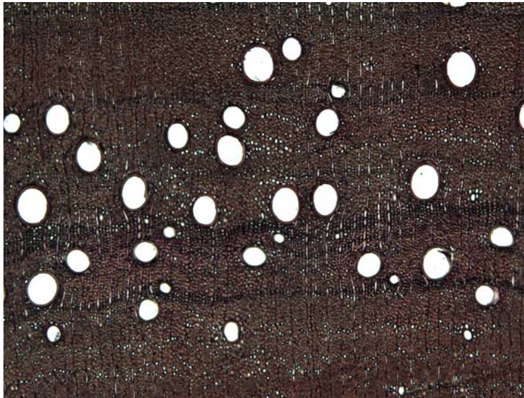
Figure 2 Transverse section of Guaiacum officinale showing a lack of distinct growth rings (image size: 2059 \mu\text{m} wide by 1544 \mu\text{m} tall). Photo: A Wiedenhoef.
