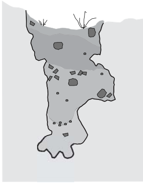
Figure 14. Dissolution pit filled with weathered rock and soil from various filling events (Adapted from Mylroie and Carew 1995). Size of pits ranges from a few centimetres to several metres.
