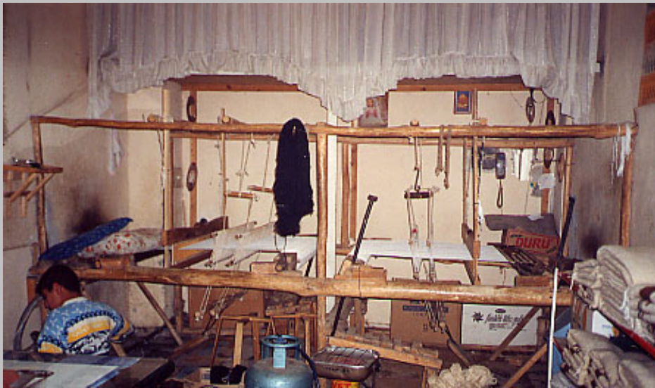
Two two-harness looms built in one frame. Siirt, Turkey. Photo: Mehmet Kiliç.
